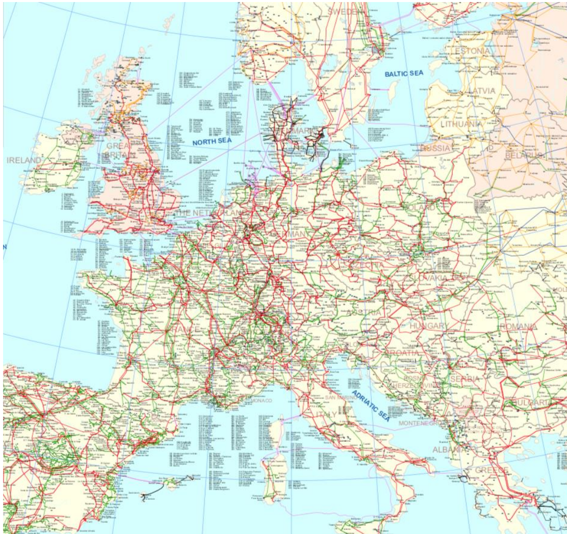
Figure 1 – Existing high voltage power network in Europe (red is 380 kV, green is 220 kV) (ENTSO-E, 2023)
