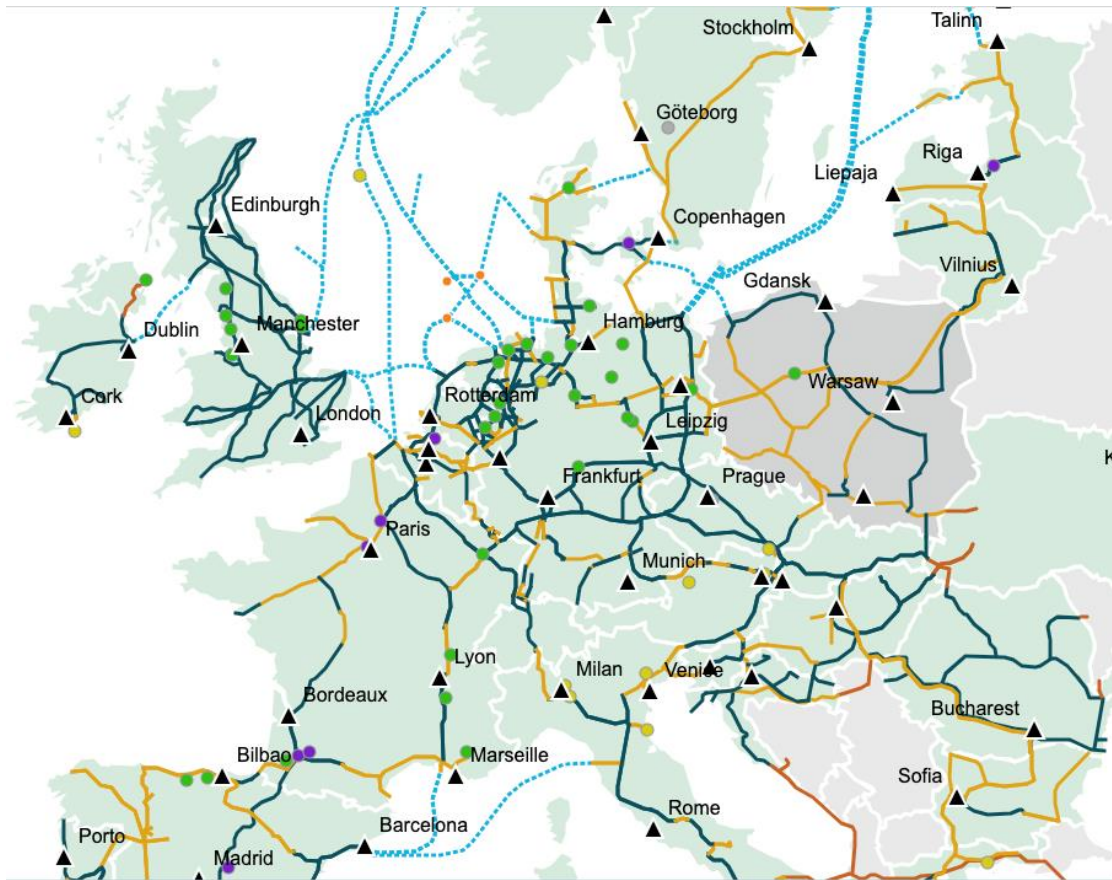
Figure 2 – European Hydrogen Backbone. Green lines are repurposed, existing natural gas infrastructure, yellow and orange lines are to be developed (EHB, 2023).
